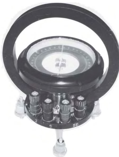
Fig 3.13 Tangent galvanometer (This diagram need not be drawn in the examination)
